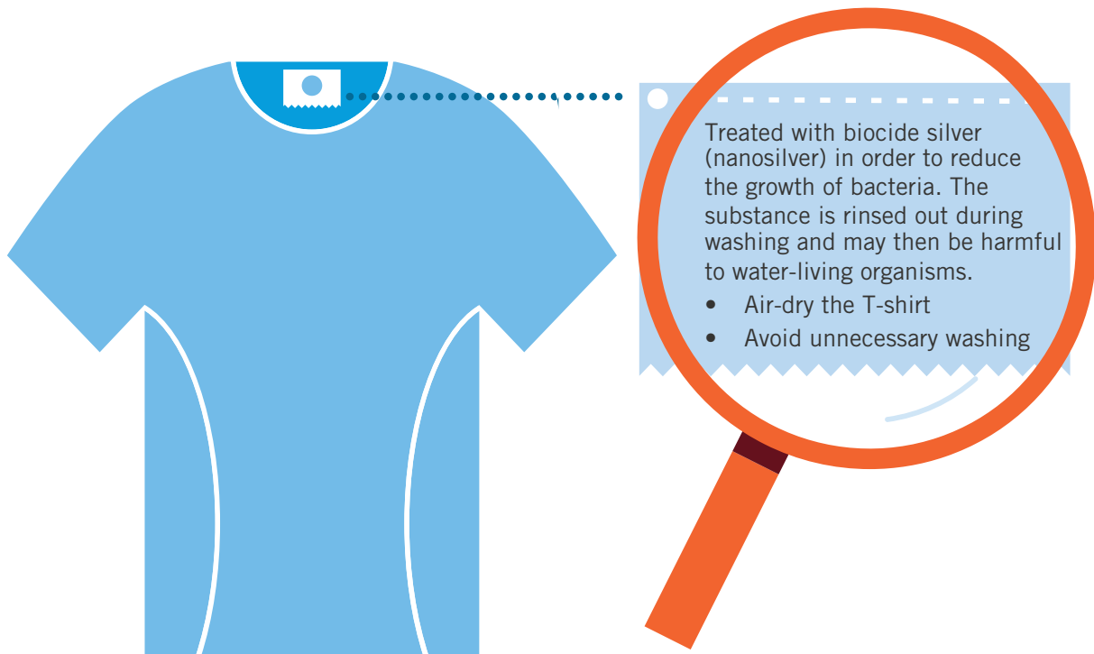
Examples of labelling on a shirt treated with a silver salt in order to avoid bad smell.
