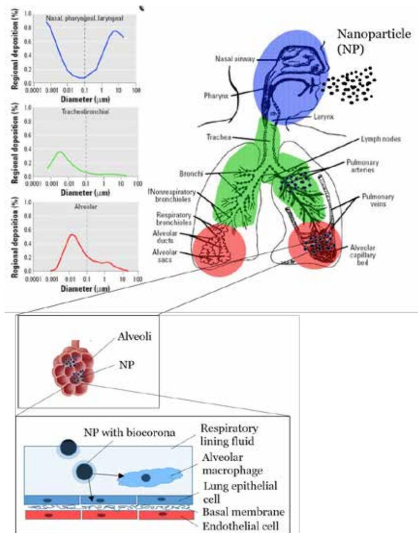
**Figure 1.** A schematic representation of nanoparticle deposition and interaction with the respiratory lining fluid. The image is reproduced version from Oberdörster et. al., 2005. [26].
