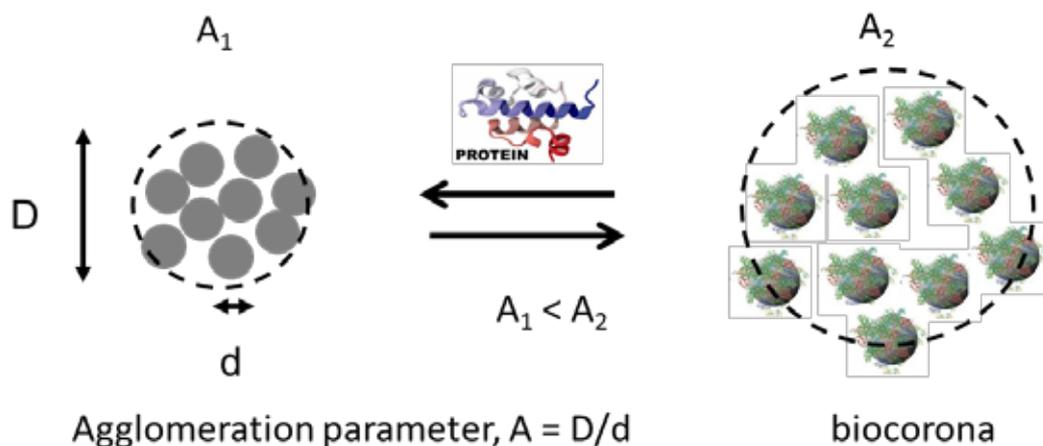
**Figure 2.** The agglomeration of nanoparticles is described by the agglomeration parameter, which distinguishes soft from hard agglomerates. Adsorption of biomolecules in the respiratory lining fluid can affect the inter-particle interaction by e.g. changing the nanoparticle surface charge and screening van der Waals bonding that weakens their interaction.
